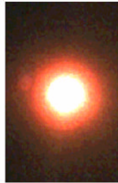
Condenser's annular ring image formed at the intermediate image plane of objective
