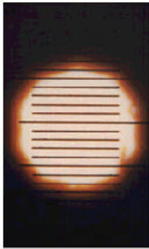
Objective micrometer placed on sample stage Nikon Optiphot Plan 40x/0.55 objective, N.A. 1.25 Phase condenser
